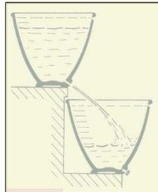
Principle of a water clock for
